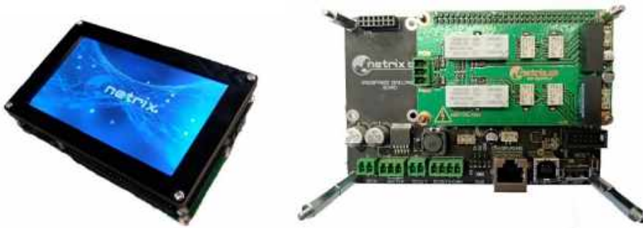
Fig. 1. Module with FT811 display and STM32H7 microcontroller and high voltage converter module
