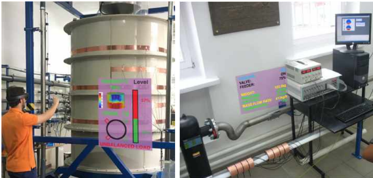
Figure 1. Holographic visualization of important flow parameters extracted from ECT measurements. Left: Silo container feeding parameters seen as by holographic HMD operator. Right: holographic display of the vital parameters of pneumatic conveying of bulk solids within a pipeline.
