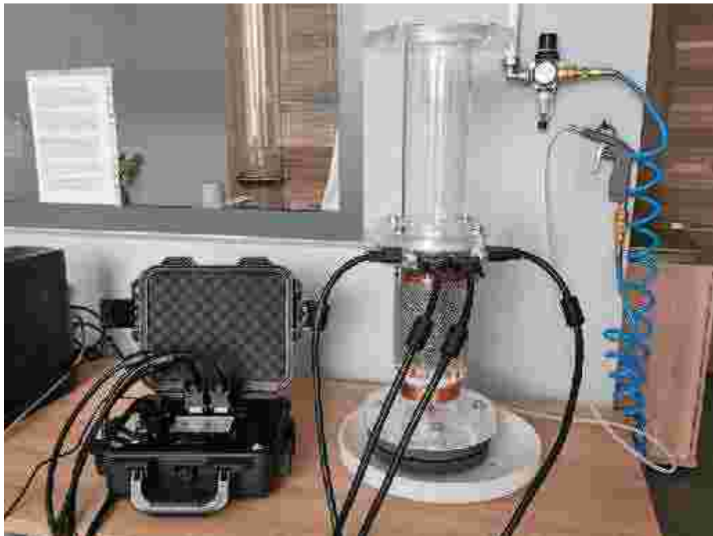
Fig. 3. Mesh sensor on the test stand
