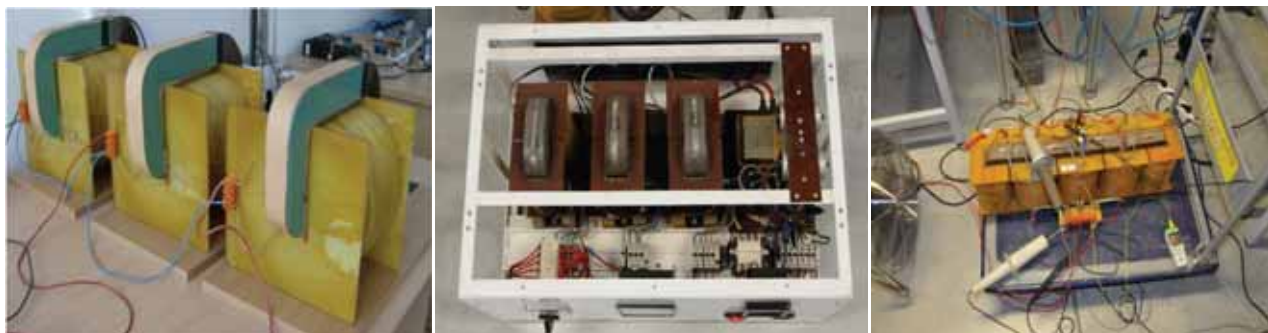
Fig. 1. Power supplies for a sliding discharge plasma reactor: a) transformer power supply, b) integrated power supply, c) five-column power supply
