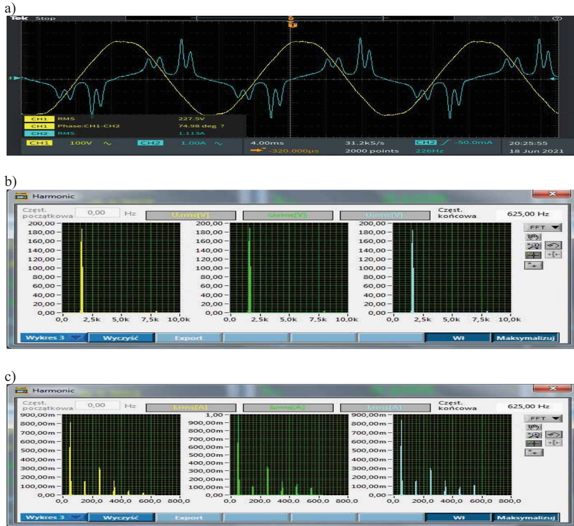
Fig. 2. Results of analysis of the integrated power supply a) oscillogram of current and voltage drawn by the integrated power supply, b) THD_U , c) THD_I
