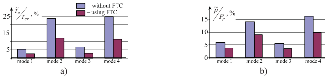
Fig. 2. The variable components of IM electromagnetic torque (a) and active power consumed from the network (b)
