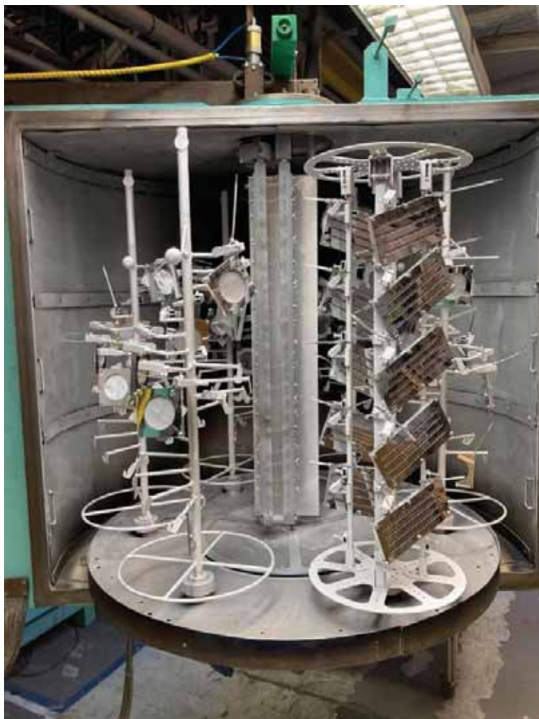
Fig. 2. Metallization technology- vacuum metallizer with samples
