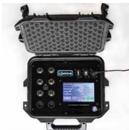
Fig. 1. The developed 64 channel reflective ultrasound tomograph
