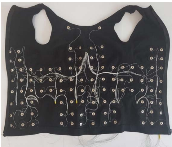
Fig. 1. Wiring of the measuring vest containing 102 electrodes
