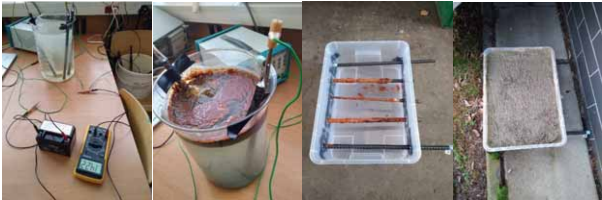
Fig. 1. Accelerated iron bar corrosion and the setup of the rebar (corroded and non-corroded) concrete slab
