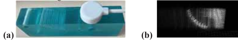
Fig. 2: Test results of the prototype tomography system: (a) – plastic phantom, (b) – reconstruction image
