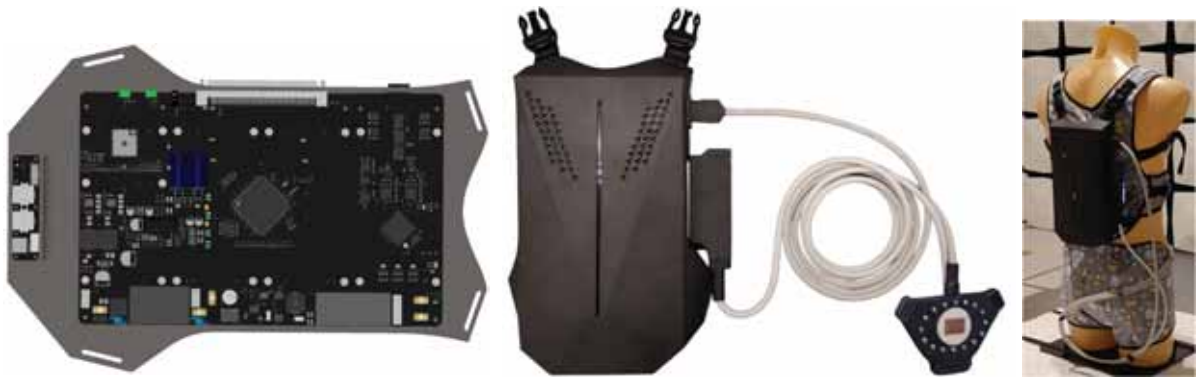
Fig. 3. UST-EIT dual tomograph for bladder monitoring
