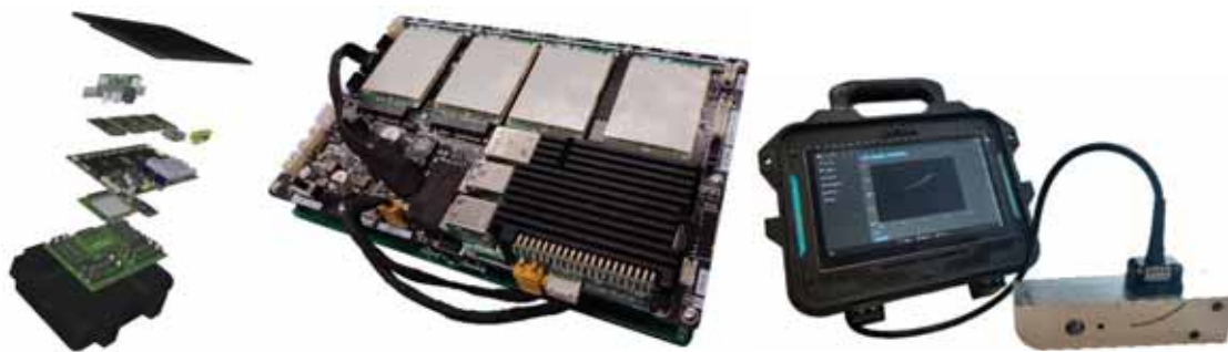
Figure 1. Defectoscope beamforming tomograph. Hardware project, construction and final product
